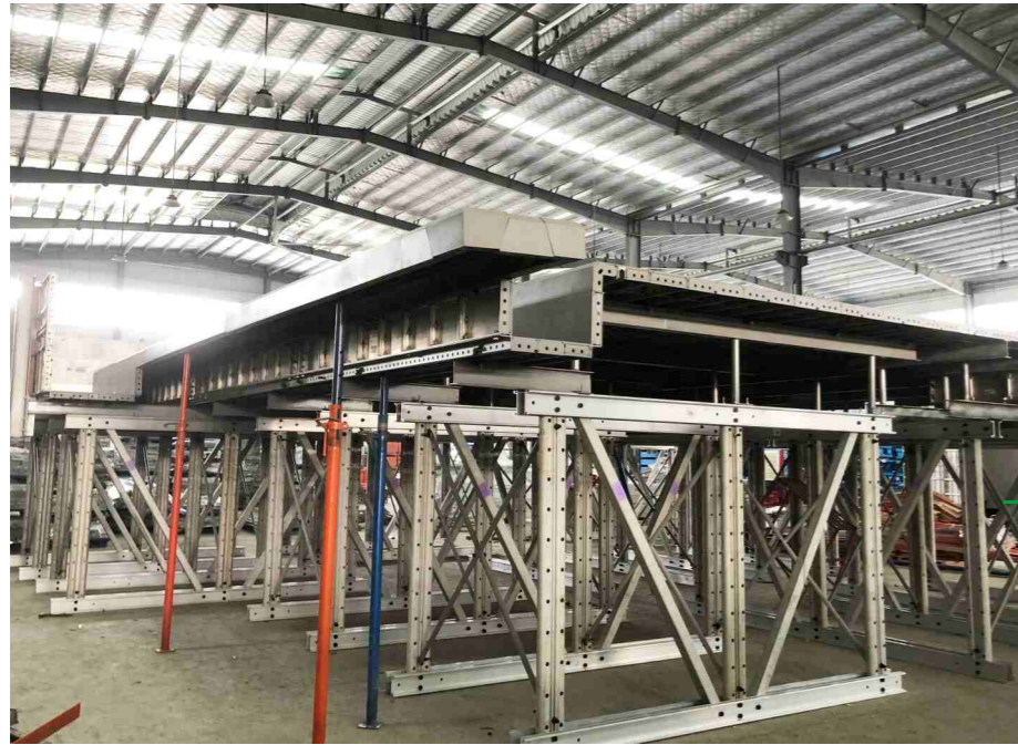
TRUSS-TYPE TABLE FORMWORK 桁架式台模
